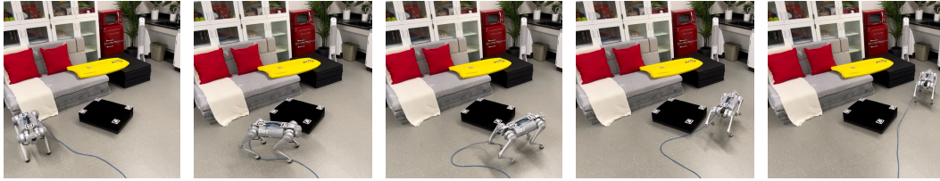
Figure 9: This figure illustrates the robot’s moving skill, the robot reaches the target location while avoiding an obstacle on the path. The collision-free trajectory is generated by an informed RRT* path planner.
