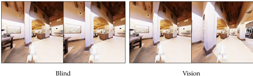
Figure 7: Comparison between Go2 blind policy and vision policy. The blind policy failed to avoid the obstacles and got stuck. The vision policy detected the obstacle and got around to avoiding it.
