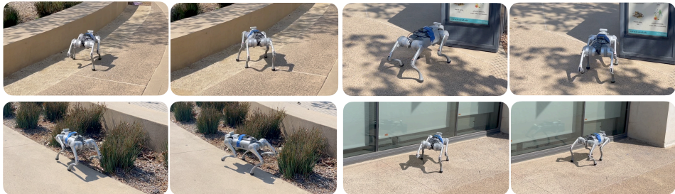
Figure 9: Obstacle avoidance screenshots. Locomotion policy can ensure collision-free in the face of high grass, certain transparent glass, and large objects under strong sunlight. The policy presents robustness on sand and grass terrains.
