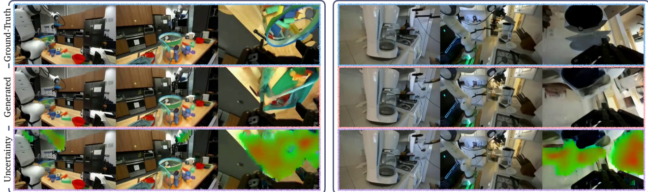
Figure 12. VidPlan localizes uncertain regions with objects morphing or disappearing. (Left) The video model deforms the cylindrical bars and other objects in the bag, which corresponds to areas of high uncertainty. (Right) Similarly, the video model is uncertain about its hallucinations of the lid of the coffee maker disappearing in the wrist-camera video.
