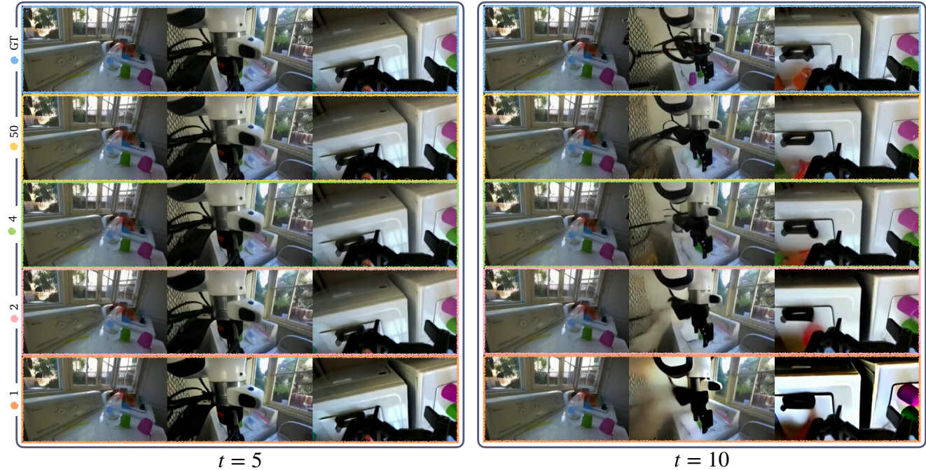
Figure 17. Flow map model rollouts at t = 5 and t = 10 for different numbers of denoising steps. Across all models, video generation quality does not noticeably degrade at t = 5 . However, the background quality degrades moderately for the 1-step and 2-step models at t = 10 , unlike the 4-step model.
