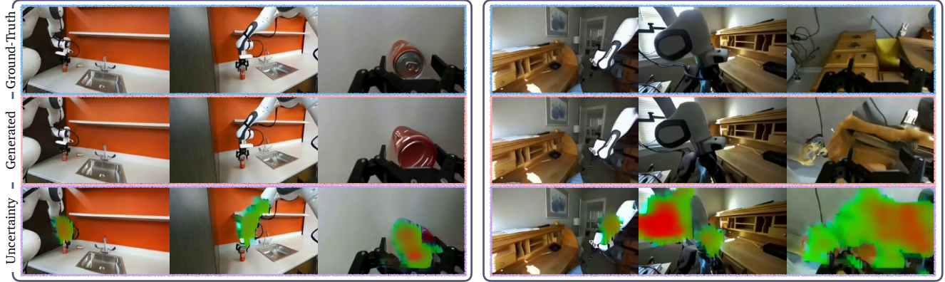
Figure 14. VidPlan identifies non-physically-consistent future predictions. In the generated videos, the video model morphs the soda can and the drawer chest. VidPlan localizes these hallucinations in the composited uncertainty maps.
