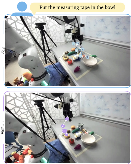
Figure 8. Sample action trajectory from \pi_{0.5} and VidPlan in the measuring tape task. (Top) \pi_{0.5} does not follow the instruction and takes a convoluted path that first pushes the penguin before putting the mug in the bowl. (Bottom) Via inference-time planning, VidPlan goes directly towards the measuring tape guided by the reward model.
