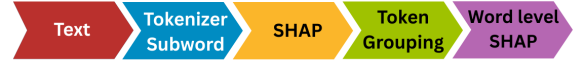
Figure 2: Word-level SHAP aggregation pipeline. Token-level SHAP values produced by a transformer model are grouped into words based on tokenizer boundaries and text alignment, then aggregated to produce interpretable word-level attributions.
