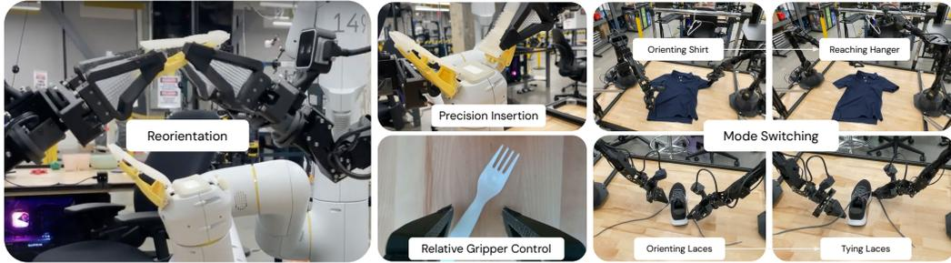
Figure 4: *Learned Behaviors*. We observe interesting behaviors the model is able to learn from the data, including reorientation and precision insertion in FingerReplace, relative gripper control in RandomKitchen, and mode switching behaviors in ShirtMessy and LaceMessy.
