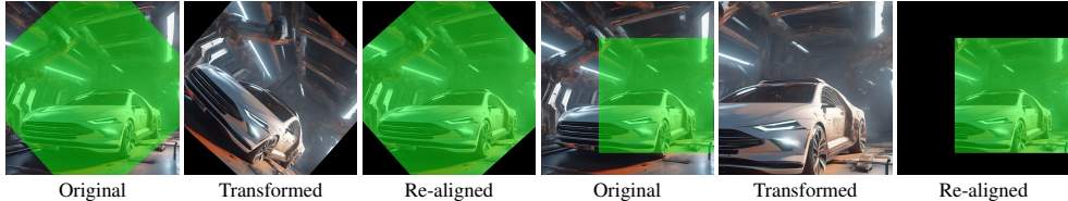
Figure 8: Estimation and alignment of geometric attacks. In green: the masked area used for cosine similarity.
