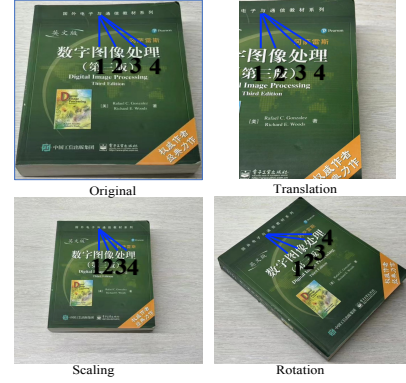
Figure 5: The relative sequence of inliers does not change freely with translation, scaling, and rotation.
