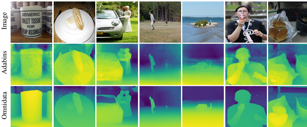
Figure 8: Comparisons of estimated depth maps that generated by Adabins (Bhat et al., 2021) and more advanced Omnidata (Eftekhari et al., 2021). We visualize the depth maps in color for better comparisons.
