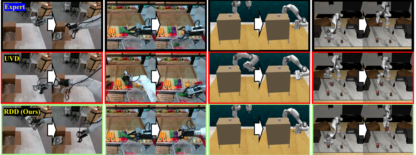
Figure 4. Qualitative results of RDD and UVD functioning on both real-world (AgiBotWorld) and simulation (RLBench and LIBERO) benchmarks. Blocks outlined in black are sub-tasks decomposed by the same task-specific heuristic used in the visuomotor policy’s training set; blocks outlined in green are sub-tasks found by RDD; and blocks outlined in red are sub-tasks found by UVD.
