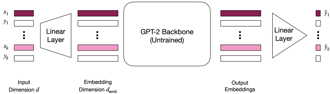
Figure 14: TART reasoning module architecture. The reasoning module takes as input sequences of (x, y) pairs of dimension d . A linear layer is used to project d to the hidden dimension size of the GPT-2 backbone. Finally, a linear layer is applied to the outputs of the backbone to generate predictions for each x_k in the input sequence.
