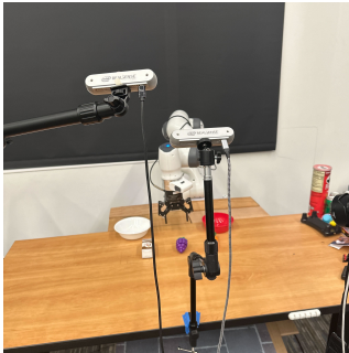
Figure 5: The camera angle invariance setup: old camera on the right, new camera angle on the left.
