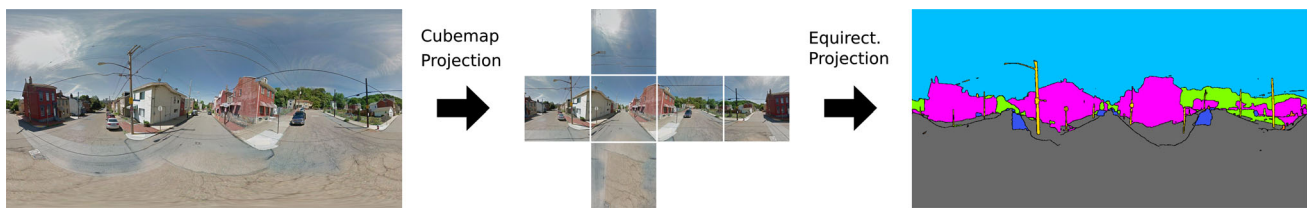
Fig. 7 The processes of automatic semantic mask generation. As a first step, we generate cubemaps of panorama and then generate a mask of each cubemaps by the state-of-the-art CNN model. As the last step, we project a mask of cubemaps to panorama
