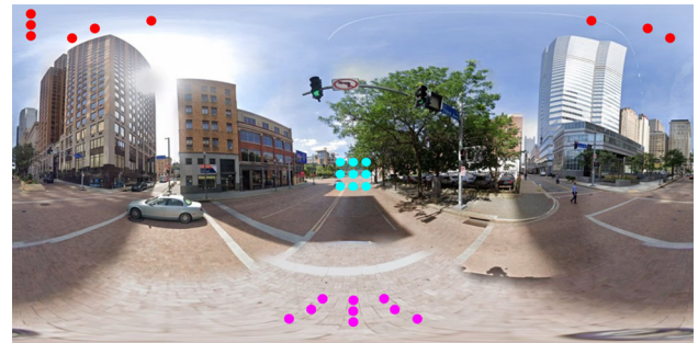
Fig. 4 The offsets of spherical convolution. Three different kernel positions are shown to highlight the differences between offsets. On the equator, kernel maps the neighboring pixels. As we approach to the poles, the deformation gets bigger. When the borders are exceeded, the points are taken from the other side of the 360° image
