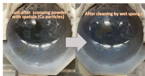
Fig. 4: Snap of mortar before and after wet sponge cleaning.
