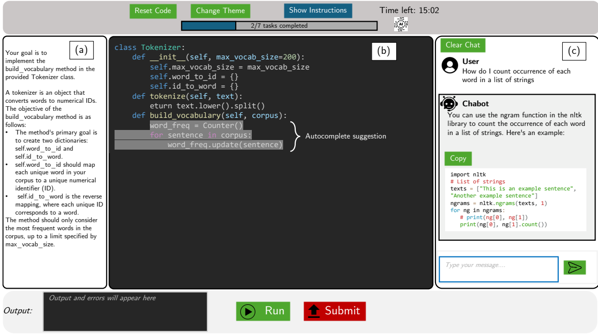
Figure 2: We introduce RealHumanEval , an online evaluation platform for LLM-assisted coding. The platform consists of (a) a customizable task description, (b) the code editor which shows autocomplete suggestions in grey, and (c) the chat assistant. Above the editor, users can check their task progress and the amount of time left, reset the editor, change the editor theme, and view study instructions. Below the editor, they can run and submit their code.
