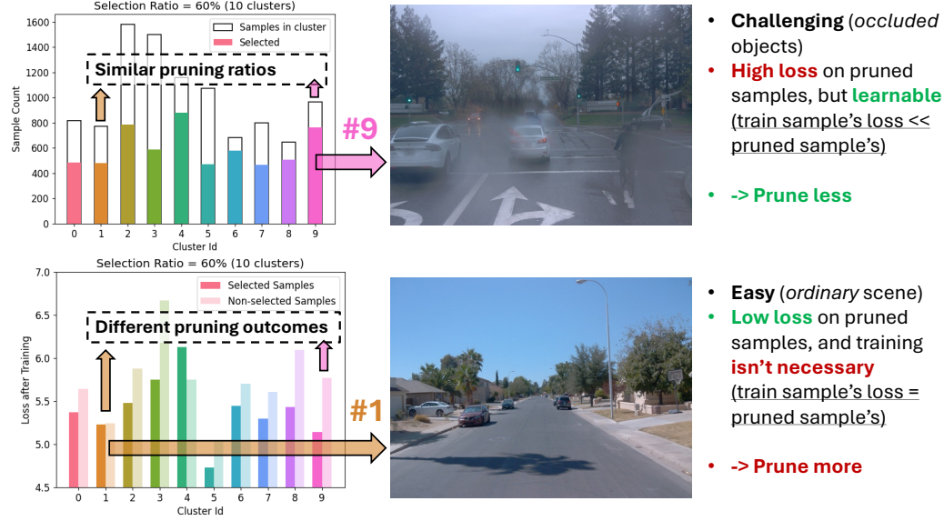
Figure 1: Illustration on density-based data pruning (Shen et al., 2025) with 10 clusters on Waymo Dataset, retaining 60% of images. Samples in each clusters generally corresponding to different semantic/scenarios (e.g., rainy urban roads for cluster #9 ( Top Right ), clear residential neighborhood for cluster #1 ( Bottom Right )). For a global uniform pruning threshold (e.g., removing the sample if there exist other samples within some threshold radius of r on visual embeddings). Samples in different clusters are pruned with different ratios due to the different level of visual similarity ( Top Left ). Training a proxy model on the pruned data, Bottom Left shows the analysis of the trained model's loss on kept vs. pruned samples within different clusters. Clusters like #1 show pruned samples having lower/comparable loss to kept ones, suggesting redundancy. Conversely, clusters like #9 exhibit significantly higher loss on pruned samples, indicating that valuable, non-redundant information was discarded. This inherent heterogeneity in data motivates ADADEDUP's adaptive approach. Our work, ADADEDUP, addresses this by synergistically integrating density-based pruning with model-informed feedback at a cluster-adaptive level; it first performs an initial pruning and then uses signals from a proxy model to adaptively refine pruning intensity for each cluster.
