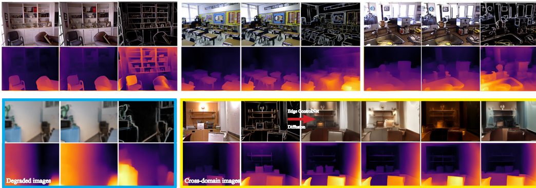
Figure 1: Depth visualizations on NYU-v2 Silberman et al. (2012). For each triplet in the first row, we showcase the RGB image, the edge-highlighted map, the edge map, and their corresponding depth maps predicted by pre-trained DPT Ranftl et al. (2021). The edge maps are obtained using the hybrid edge detection strategy. In the second row, we show more edge observations in degraded images or cross-domain applications.
