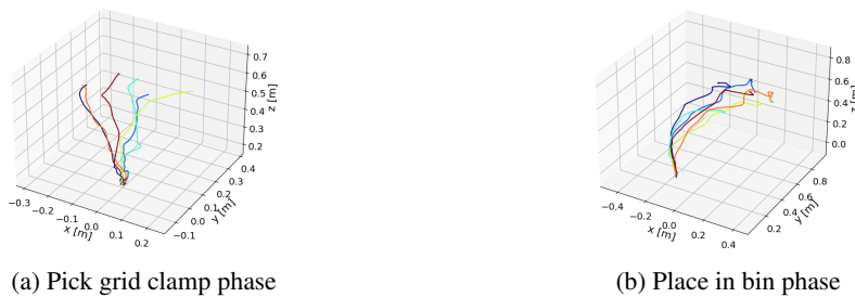
Figure 3: 3D position plots of 6 kinesthetic demonstrations of self-organising workstation task in the object frame, described in 3
