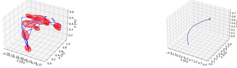
(a) Learned GMM Model (means and covariances in red) from object-centric demonstrations (blue) (b) Object-centric trajectory with vanilla KMP (not adapted)
