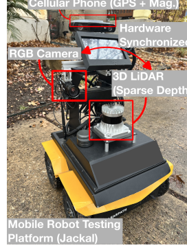
Fig. 7: Mobile robot, Clearpath Jackal, used for real-world experiments with sensors for deployment annotated.
