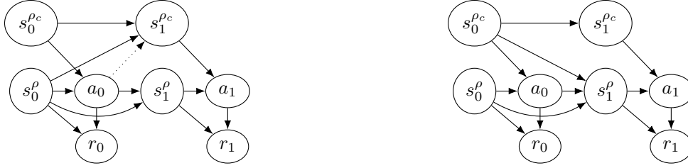
Figure 1: (Left) Reward-relevant/irrelevant factored dynamics of (Zhou, 2024b). (Right) Exogenous-Endogenous MDP model of (Dietterich et al., 2018). The dotted line from a_t to s_{t+1}^{\rho_c} indicates the presence or absence is permitted in the model.
