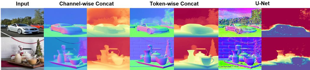
Figure S2: Depth and normal estimation multi-task visualizations comparing channel-wise concatenation, token-wise concatenation, and U-Net are shown. While channel-wise concatenation often leads to suboptimal performance and U-Net struggles with multi-task learning, DICEPTION effectively generates high-quality outputs for multiple tasks.
