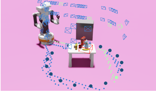
Fig. 3: Example scene with sampled candidate paths (blue) for the robot pose towards the target object (red box). The paths consist of SE(2) poses for the base and SE(3) poses for the head-mounted camera (visualized from the robot to the base goals). The current optimal path is highlighted in green.
