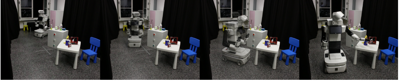
Fig. 1: Real-world execution of our active perception and grasping pipeline. The mobile manipulator robot, equipped with a head-mounted camera, efficiently explores the scene to detect grasps on the target object and effectively performs the grasp by evaluating its executability. Video demonstrations are provided at our project website: sites.google.com/view/actpermoma .
