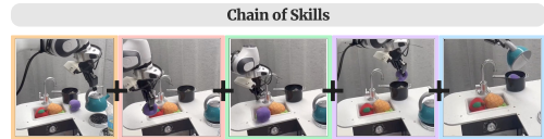
Figure 8: Illustration of zero-shot skill chaining. We demonstrate executing five skills in sequence, creating hard OOD setups.
