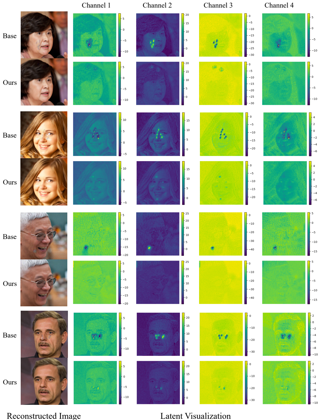
Figure 14. Visualization of MCLC’s suppression of blob artifacts. The base solver is LDPS and the task is Gaussian deblurring.
