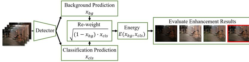
Figure 4: The pipeline of our proposed LIME-Eval.
