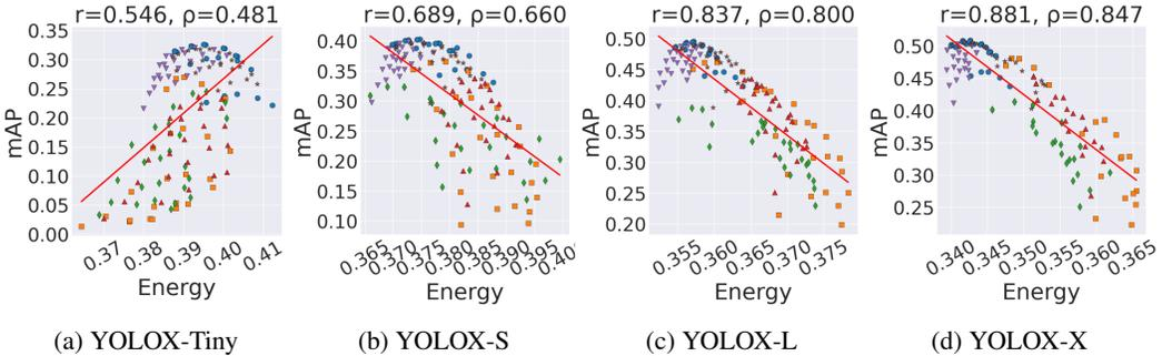
Figure 7: Energy versus mAP under different base detectors on our synthesized dataset.
