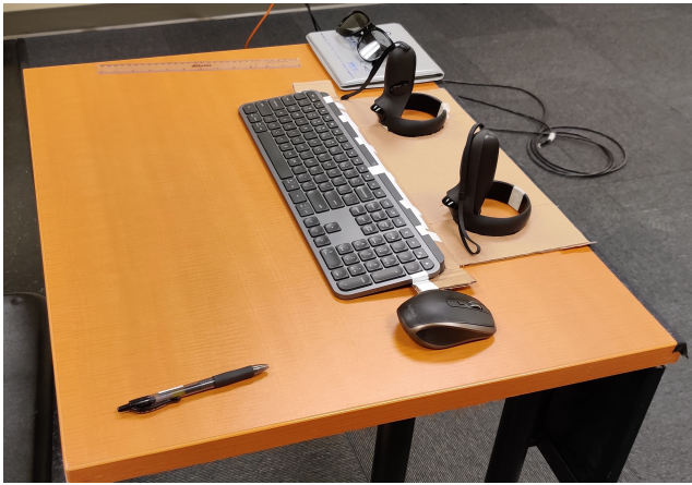
Figure 5: The controllers, normally held in the user's hands, are placed in a cardboard template, allowing the headset to deduce the location of the physical keyboard.
