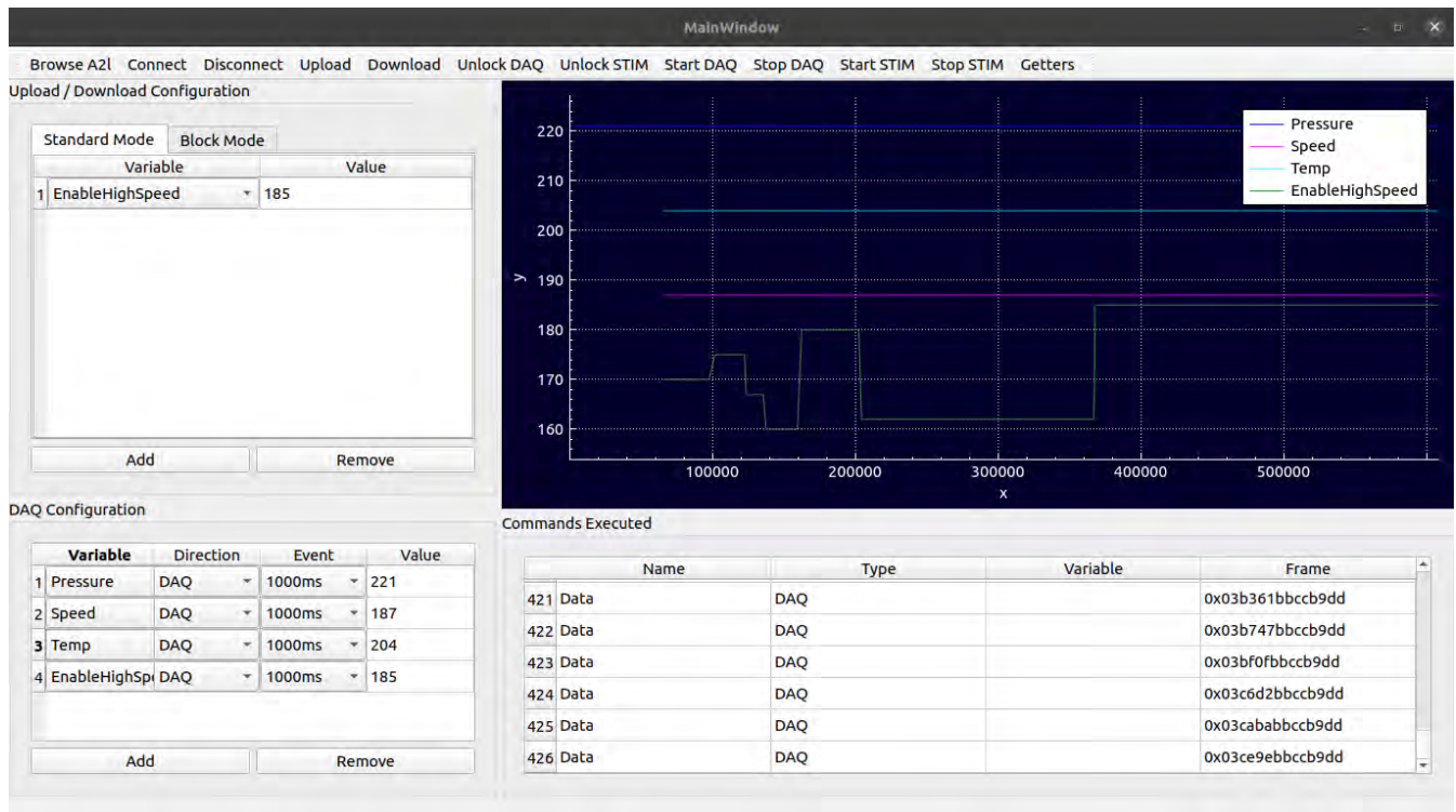
Fig. 4. Data acquisition while making calibration to one of the measured variables at the same time using Multi-core XCP.
