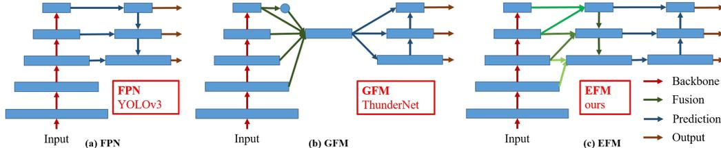
Figure 6: Different feature pyramid fusion strategies. (a) Feature Pyramid Network (FPN): fuse features from current scale and previous scale. (b) Global Fusion Model (GFM): fuse features of all scales. (c) Exact Fusion Model (EFM): fuse features depend on anchor size.
