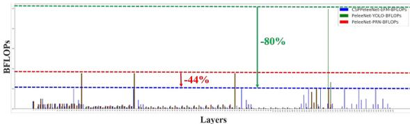
Figure 7: Computational bottleneck of PeleeNet-YOLO, PeleeNet-PRN and CSPPeleeNet-EFM.
