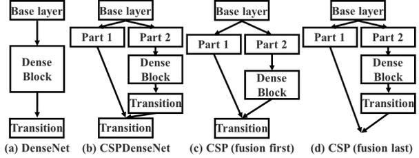
Figure 3: Different kind of feature fusion strategies. (a) single path DenseNet, (b) proposed CSPDenseNet: transition  $\rightarrow$  concatenation  $\rightarrow$  transition, (c) concatenation  $\rightarrow$  transition, and (d) transition  $\rightarrow$  concatenation.
