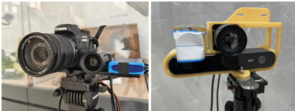
(a) Our designed hybrid imaging system. (b) RGB-T and RGB-D imaging system.
