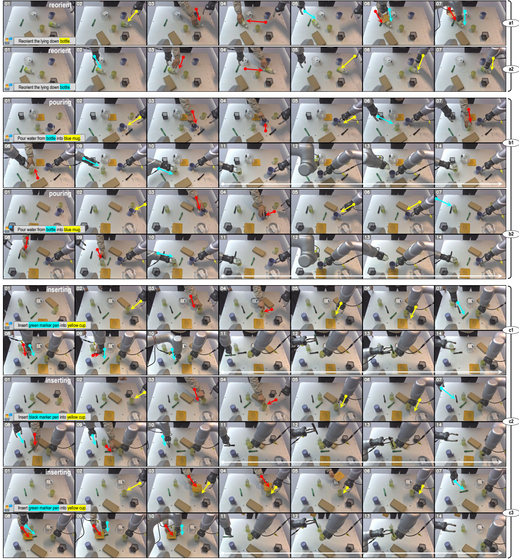
Figure 16: Visualization of test results for VLBiMan’s robustness performance in cluttered scenarios. We selected three tasks, reorient (corresponding to examples a1/a2 ), pouring (corresponding to examples b1/b2 ), and inserting (corresponding to examples c1/c2/c3 ), for extensive evaluation. In these examples, there are not only various irrelevant objects that can easily lead to semantic ambiguity and execution obstacles , but we will also unexpectedly rearrange the target object during the pre-grasping stage. This requires the VLBiMan to be able to quickly and nimbly find the target object again from the cluttered scene based on the task’s linguistic instructions. This process faces many significant non-trivial challenges. The red arrow indicates the direction of the manually moved or deliberately obscured object (interfering). The cyan arrow and yellow arrow indicate the movement direction of the left and right robotic arms (chasing) respectively.
