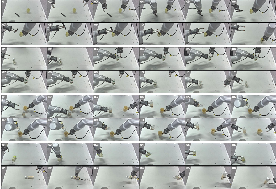
Figure 12: Examples of four transferred bimanual tasks with synchronized dual-arm movement. Segments from top to bottom are tasks inserting , unscrew , and pouring , which have relatively high dual-arm synchronizability. The last row are examples of single-arm task reorient , explicitly examining left- or right-handed execution strategies.
