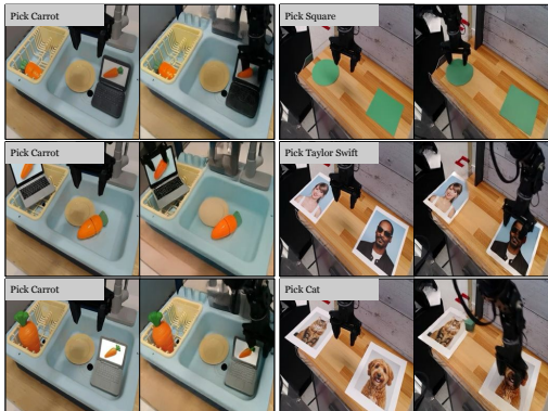
Figure 10: OOD: Failure modes. Left: We add a laptop to the scene, which displays an image of a carrot. In 15% trials, OpenVLA grabs the laptop instead of the real carrot. Right: We test the ability distinguish to between squares and circles, celebrity faces, and cats and dogs, with all policies scoring near-chance.
