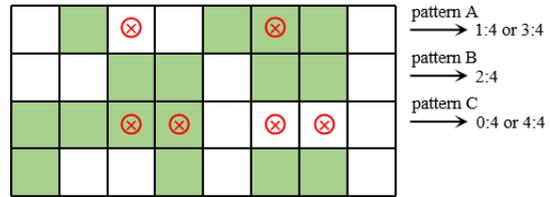
Figure 2: Three patterns of X:4.  $\otimes$  represents different weight choices of 50% unstructured and a 2:4 pattern.
