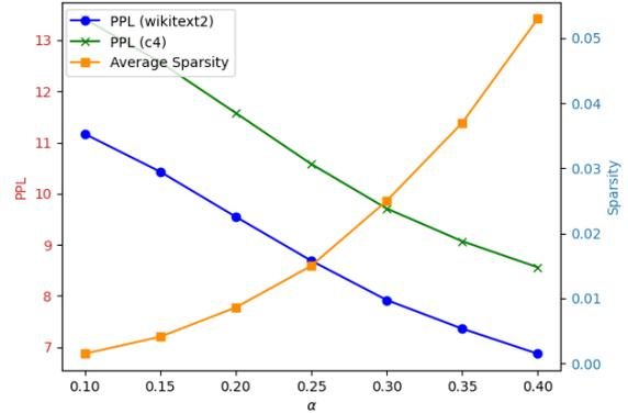
Figure 3: Exploring the impact of factor  $\alpha$  on model perplexity and the average sparsity of recover weight in LLAMA2-7B.
