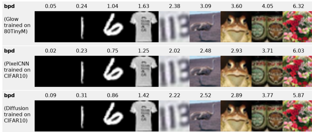
Figure S1: Visualization of the bits-per-dimension (bpd) measure for image complexity, sorted from low to high. Image samples are taken from MNIST, Fashion-MNIST, CIFAR10 and CIFAR100, in addition to a completely black image sample. bpd is calculated from the density produced by a Glow (Kingma & Dhariwal, 2018) model pretrained on 80 Million Tiny Images, a PixelCNN model trained on CIFAR10, and a diffusion model trained on CIFAR10.
