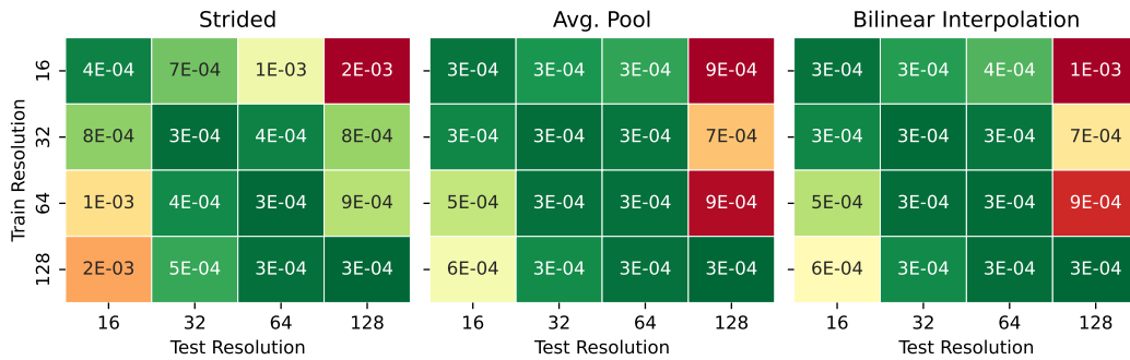
Figure 47: FNO on Darcy with varied data downsampling strategies. FNO is trained and tested on data that is downsampled via from the max resolution of 128 via three strategies: strided downsampling, average pooling, and bilinear interpolation. On average FNO incurs higher losses across test resolutions that differ from the train resolution across all three downsampling strategies.
