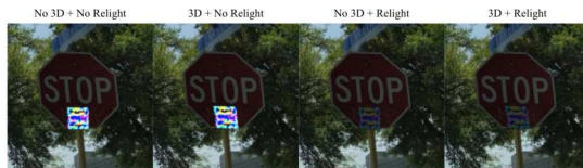
Figure 3: The rightmost stop sign has a patch rendered with a perspective and relighting transform making it more realistic. The first and second images have patches that are too bright whereas the first and third images have patches that do not respect the sign’s orientation.
