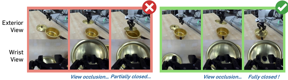
Figure 6: Qualitative results on real-robot manipulation task . Under partial-view occlusion at the wrist view, the baseline model (left) fails to align the lid with the pot, resulting in inaccurate placement. In contrast, RS-CL (right) achieves precise alignment and successful closing by effectively incorporating proprioceptive state information into its representation.
