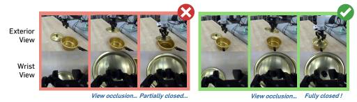
Figure 6: **Qualitative results on real-robot manipulation task.** Under partial-view occlusion at the wrist view, the baseline model (left) fails to align the lid with the pot, resulting in inaccurate placement. In contrast, RS-CL (right) achieves precise alignment and successful closing by effectively incorporating proprioceptive state information into its representation.
