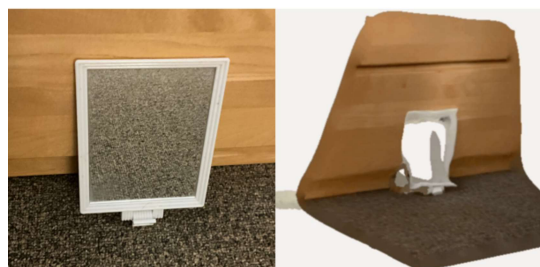
Fig. 1. Mirror Reconstruction with Conventional LiDAR. Conventional LiDAR systems fail to map the 3D shape of mirrors because mirrors reflect light away from the sensor. As a result, holes appear in the reconstruction.
