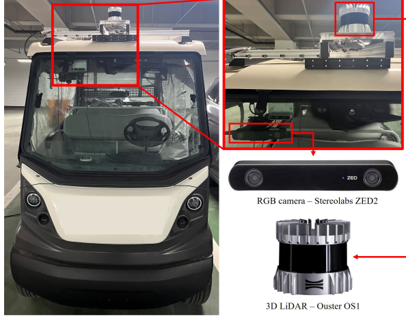
Figure 4. Sensor setup for the custom dataset collection.
