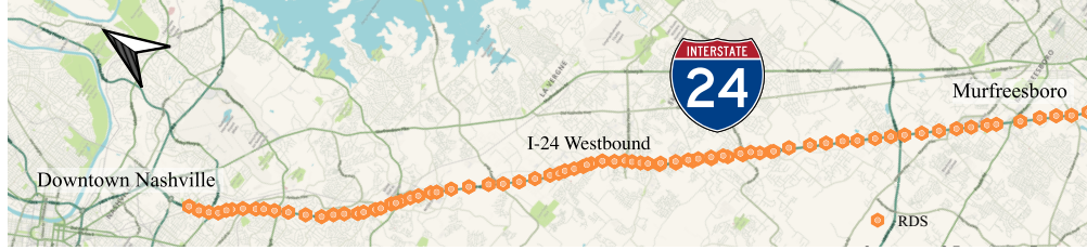
Figure 1: Map of the Radar Detection Systems (RDS) sensor network deployed for data collection. 49 RDS sensors are deployed along Interstate 24 toward Nashville, Tennessee. Each sensor captures speed, occupancy, and volume data for each of the four lanes every 30 seconds.
