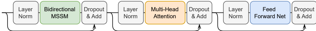
Figure 3: Stateformer: Bidirectional state space augmented transformer encoder example. It simply has an additional block prior to the attention unit with a bidirectional MSSM as seen in Equation 10.
