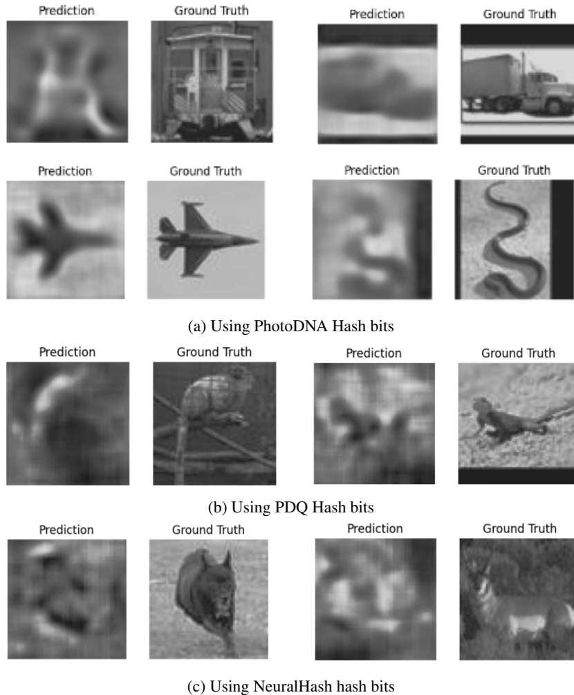
Figure 6: Samples of true STL-10 images and adversarial images generated by hash inversion attacks.
