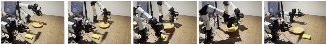
Figure 9: Real-world: “Wash the dish.” A contact-rich task involving picking up a dish and per- forming a washing motion. The policy demonstrates robustness to the dynamic forces encountered during the scrubbing interaction.
