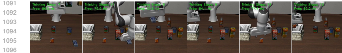
1097 Figure 13: LIBERO-Long: “Put both the cream cheese box and the butter in the basket.” A multi- 1098 step task requiring two sequential pick-and-place operations. The model increases computation at 1099 each grasp and release transition. 1100
