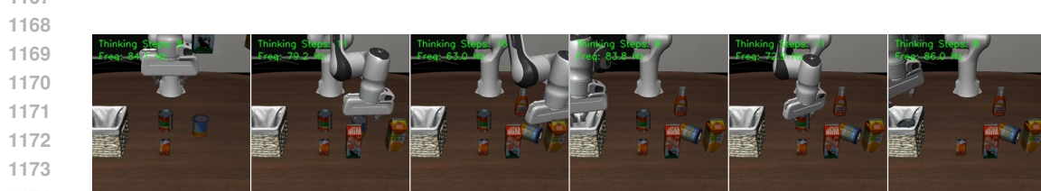
1175 1176 1177 1178 Figure 20: LIBERO-Long (failure) : “Put both the alphabet soup and the tomato sauce in the basket.” The model succeeds on the first object but fails to complete the second pick-and-place, illustrating the compounding difficulty of long-horizon multi-step tasks.
