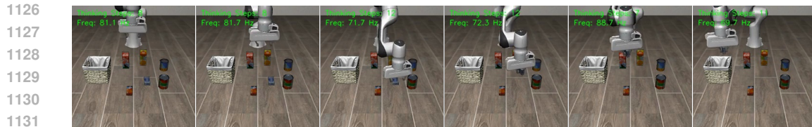
1132 Figure 16: LIBERO-Object: “Pick up the cream cheese and place it in the basket.” Similar adap- 1133 tive pattern with peak computation at the grasp point.
