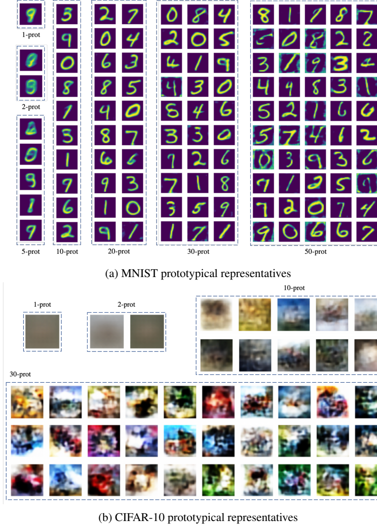
Figure 2: Exploring interpretability using synthesis from prototypes coordinates. For MNIST it is possible to observe that prototype coordinates usually reconstruct to known digits, especially with prototypes larger than 10, as we have 10 digits represented in the dataset. For CIFAR-10, one can notice that the learned clusters are gathered around role models that depict associations between foreground and background patterns, which become more detailed with the increase of the number of prototypes available for anchoring clusters.
