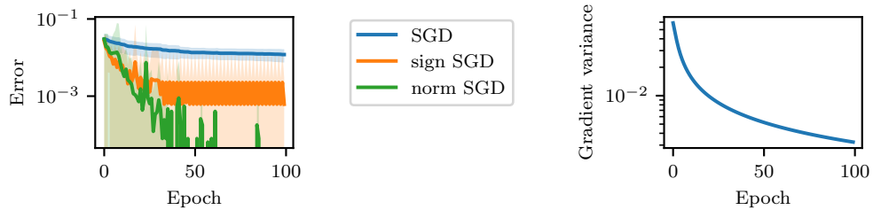
Figure 16: Left: Generalization error in the setting of Figure 15. Observe how SGD with rescaled variance (in green), an effect that can be done with SGD after adapting the learning rate, actually performs better than sign SGD (i.e., Adam with \beta_1 = \beta_2 = 0 ). Right: Variance of SGD along the training. As the training goes, SGD is losing momentum due to smaller gradient variances, hence smaller updates.
