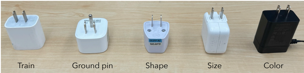
Figure 4: We test the generalization of the best-performing V1SK policy to different variations of the plug
