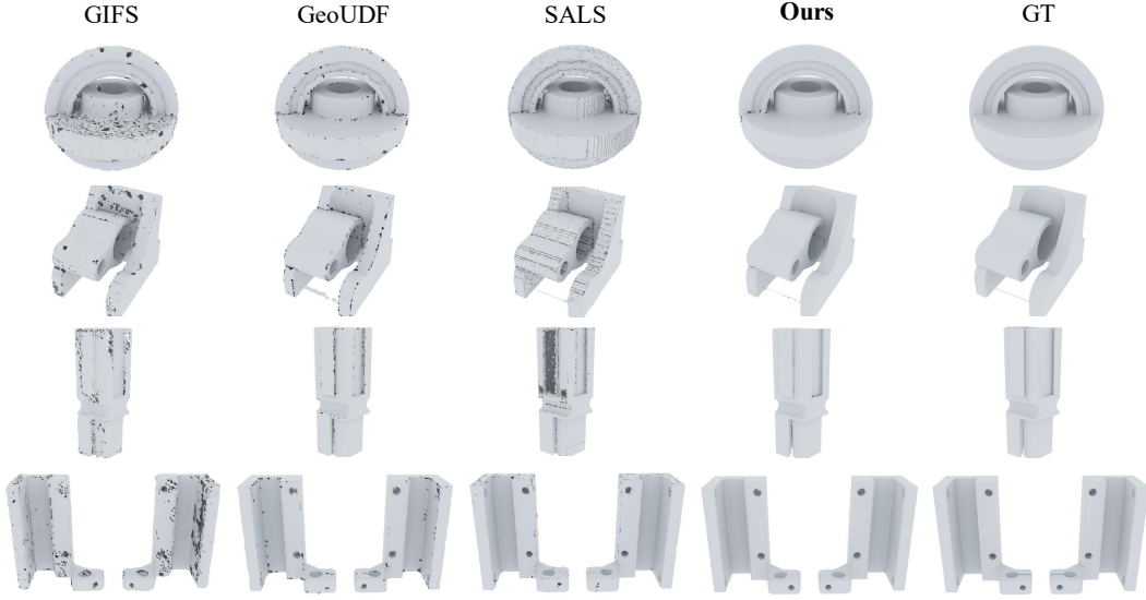
Figure 3: ABC and Non-Manifold ABC (Ren & Hou, 2025) Visualization. All methods are evaluated at a resolution of 128 with non-manifold edges preserved and holes filled. The first row shows non-manifold objects, while the subsequent three rows depict the original ABC objects.
