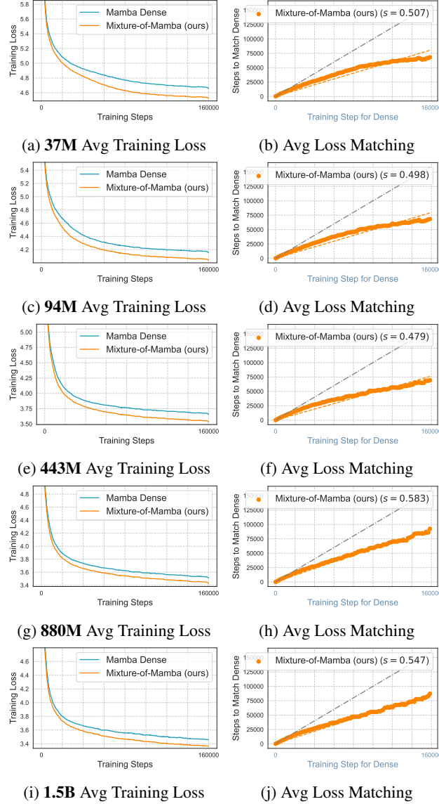
Figure 10. Average training loss and step matching plots across model scales in the Chameleon setting. Results are shown for Mixture-of-Mamba and Mamba Dense across five model scales: 37M, 94M, 443M, 880M, and 1.5B. (a, c, e, g, i) Average training loss (across image and text modalities) demonstrates consistent reductions for Mixture-of-Mamba (orange), achieving lower loss values compared to Mamba Dense (cyan) at all model scales. (b, d, f, h, j) Average loss matching plots highlight that Mixture-of-Mamba reaches the same loss values at earlier training steps compared to Mamba Dense, reflecting improved training efficiency. Overall, Mixture-of-Mamba consistently reduces average training loss and achieves more efficient convergence across all model scales in the Chameleon setting.
