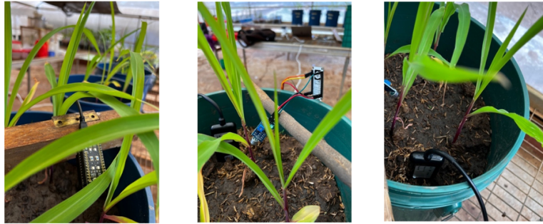
Fig. 2. Data collection using IoT sensors on Volatile Organic Compounds, microphone sensors and NPK fertilizer.
