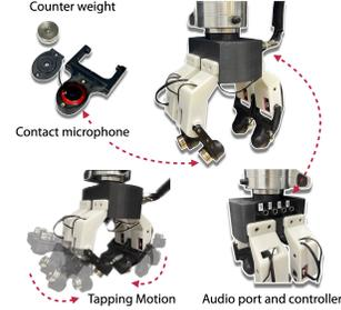
Fig. 1: Our robot hand includes four fingers where each fingertip is equipped with one contact microphone and a counterweight.
