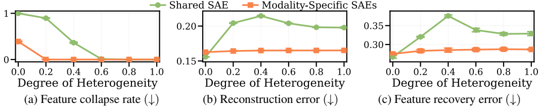
Figure 5: Comparison between a shared SAE trained on both modalities (green) and modality-specific SAEs trained separately for each modality (orange) as the cross-modal feature distance varies. Each point corresponds to SAEs trained on synthetic embeddings sampled from ground-truth feature matrices \Phi and \Psi , where the x-axis shows the cosine distance between corresponding image and text feature directions. When corresponding directions are distinct but geometrically close, the shared SAE tends to collapse them into a single learned direction, leading to higher reconstruction and feature recovery errors. In contrast, modality-specific SAEs avoid this collapse and better preserve feature directions under cross-modal feature heterogeneity, which corresponds to nonzero distance.
