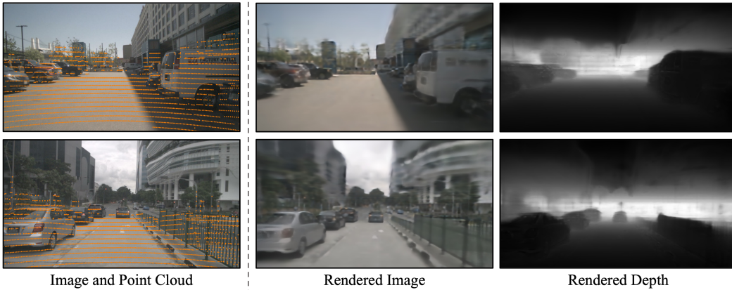
Figure 3: Illustration of the rendering results, where the ground truth RGB and projected point clouds, rendered RGB, and rendered depth are shown on the left, middle, and right, respectively.
